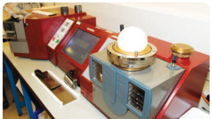
Chopin Alveograph showing stage 5 - air being pumped into dough
