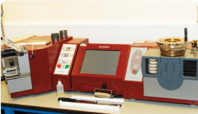
The Chopin Alveograph is a test commonly used overseas to help determine the baking potential of wheat by measuring its characteristics.
