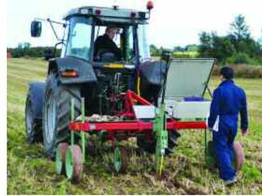
Exhaustive testing has revealed the sensor can accurately map a range of soil properties from clay to total nitrogen content, pH and cation exchange capacity.
