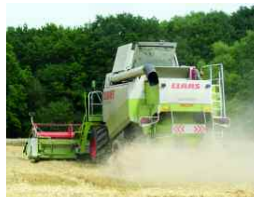
Chopping straw adds about £4-5/ha in fuel costs, but can mean more timely drilling if there's a late harvest.
