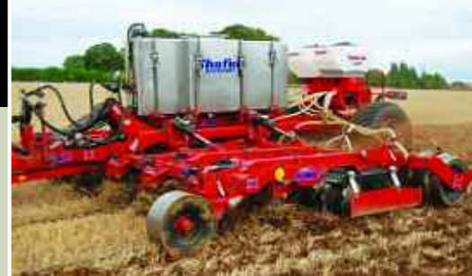
Fertiliser was placed in bands between the Trio's leading subsoiler legs and discs.
