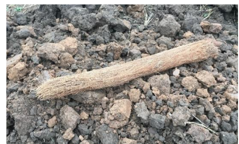
Willow roots removed from a blocked drain
