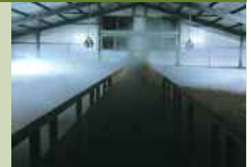
Chlorpropham (CIPC) permeates into the fabric of a store and can persist for decades.
